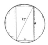
38. Stiffness of a Beam The stiffness S of a rectangular beam is proportional to its width times the cube of its depth.
